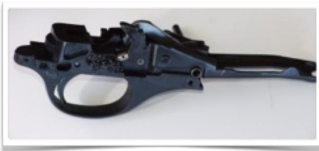
A one piece removable trigger mechanism has a simple design but effective. It can be removed by pressing out one pin on the side of the action. Whilst depressing the bolt release button pull downward on the trigger guard. We found this task easier after detaching the fore-end, barrel and bolt. We remove and clean the trigger mechanism after every 1500 rounds.
